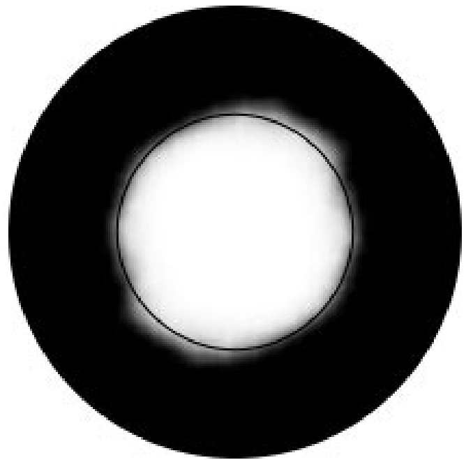
FIG. 7.—One example of the Fourier domain filter, H . Superimposed is a black ring with equivalent radius, U_H , see eq. (6). The radius of the black disk is the diffraction limit cutoff frequency.
